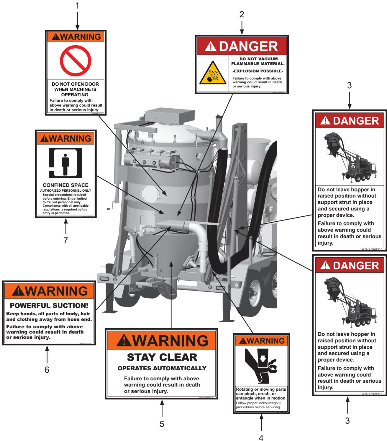
Figure 26: Hazard Identification Decals (Cont.)
